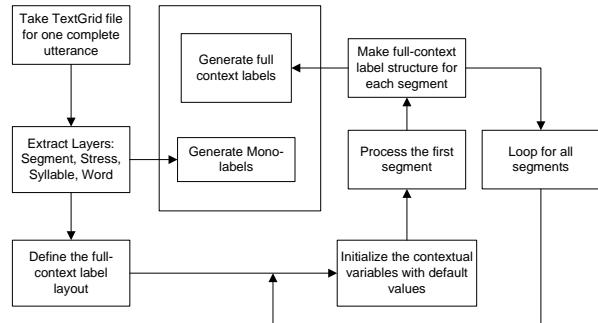
**Figure 3. Flow diagram of the HTS-format conversion utility**
