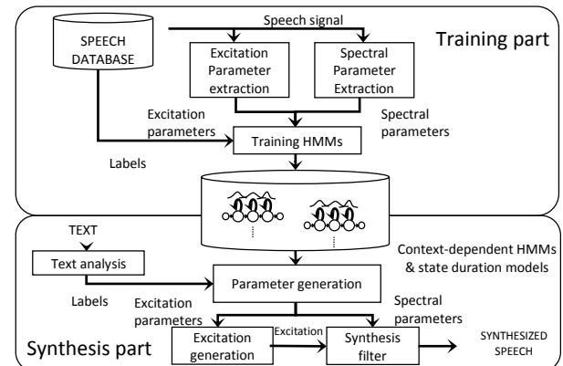
**Figure 1. Overview of Parametric speech synthesis with HMMs ([7], pp. 227)**
